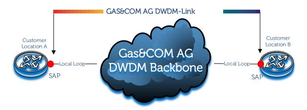
The GAS&COM DWDM Link is offered as a Single, Dual or Protected Link.
